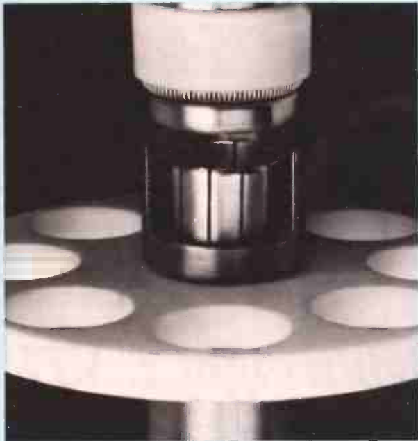
The above photo shows a cut-away view of the female connector with its built-in thermo-probe prior to its assembly with the watchband male bullet. (Note: Both the male and female connections are an integral part of the inner conductor allowing only one contact joint per section of transmission line.)
